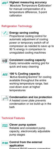
External Pt100 sensor connection for precise measurement and control directly in the external application
